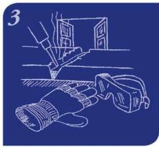
There after the granulate is soaked thoroughly with HOSCH Industruial Glue. Thereby a chemical reaction occurs. (ATTENTION! Development of heat and forming of vapours!) Wear safety goggles and gloves! Do not inhale the vapours, ventilate well!
