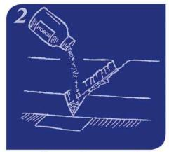
In case of extreme fractures or of lacking material as well as for the strengthening of materials the gaps and holes are filled up with HOSCH Granulate - underlay a sheet of paper to avoid trickling. Take care that the height of filling up does no exceed 2-3 mm. In case of deeper gaps or holes the filling up must be done in layers.
